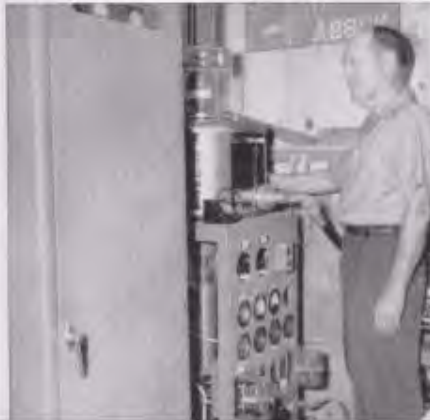
Above, the antennas at KH6UK and W1BU. KH6UK got his 28-foot Kennedy through MARS, while the eighteen-footer at W1BU came from surplus. Sam's dish tracks automatically. Below, the transmitters. Both used one-kw. klystrons by Eimac.
