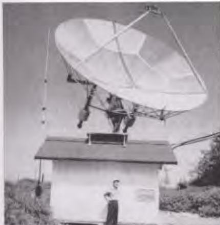
Above, the antennas at KH6UK and W1BU. KH6UK got his 28-foot Kennedy through MARS, while the eighteen-footer at W1BU came from surplus. Sam's dish tracks automatically. Below, the transmitters. Both used one-kw. klystrons by Eimac.
