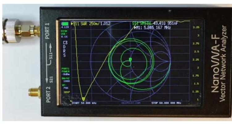
Sim Antenna This is what the circuit looks like at the end of the feed line. Notice that the SWR dips to the smallest value when it is closest to the center point (50 ohms R).
