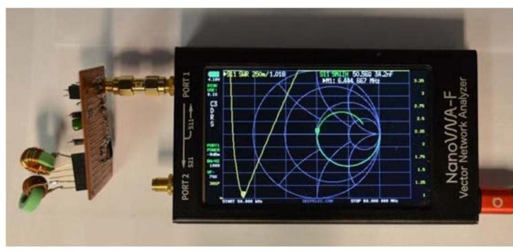
Sim Antenna The circuit consists of a Resistor, Capacitor, and Inductor in series. I also can change jumpers to change the Resistor from 50 to 100 Ohms, and bypass the Capacitor and/or the Inductor.
