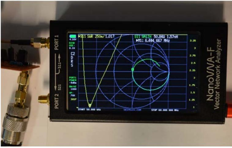
Calibration of Feed line. Sim Antenna at the end of the feed line.
